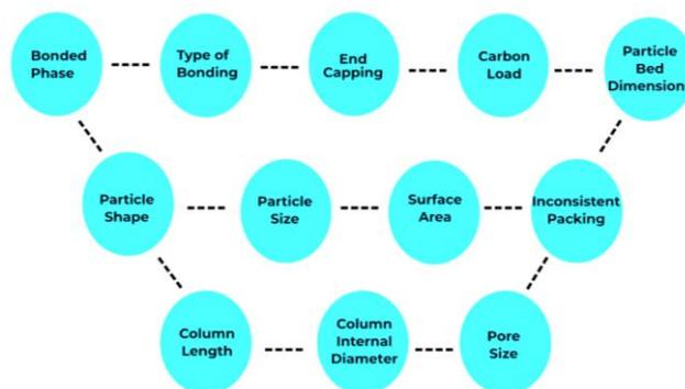
**Fig. 3.** Properties of stationary phase in column chromatography
