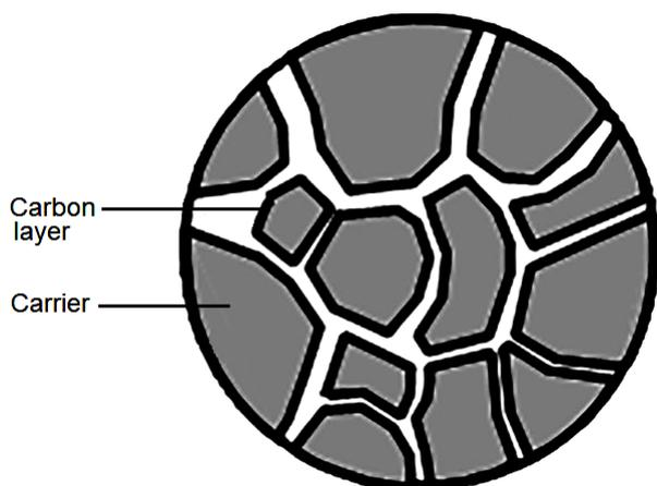
**Fig. 4.** Schematic diagram of silica-carbon composite material
