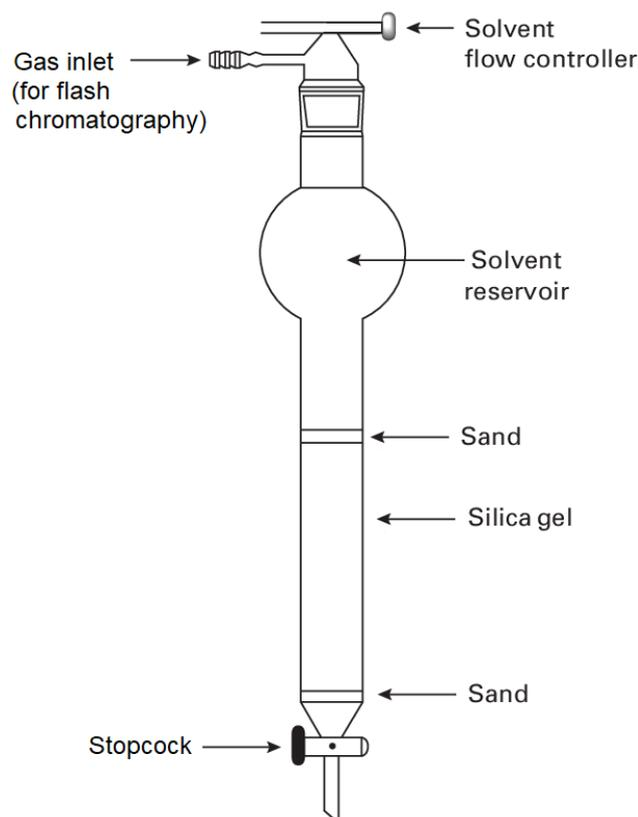
Fig. 2. Apparatus used for a typical flash chromatography
